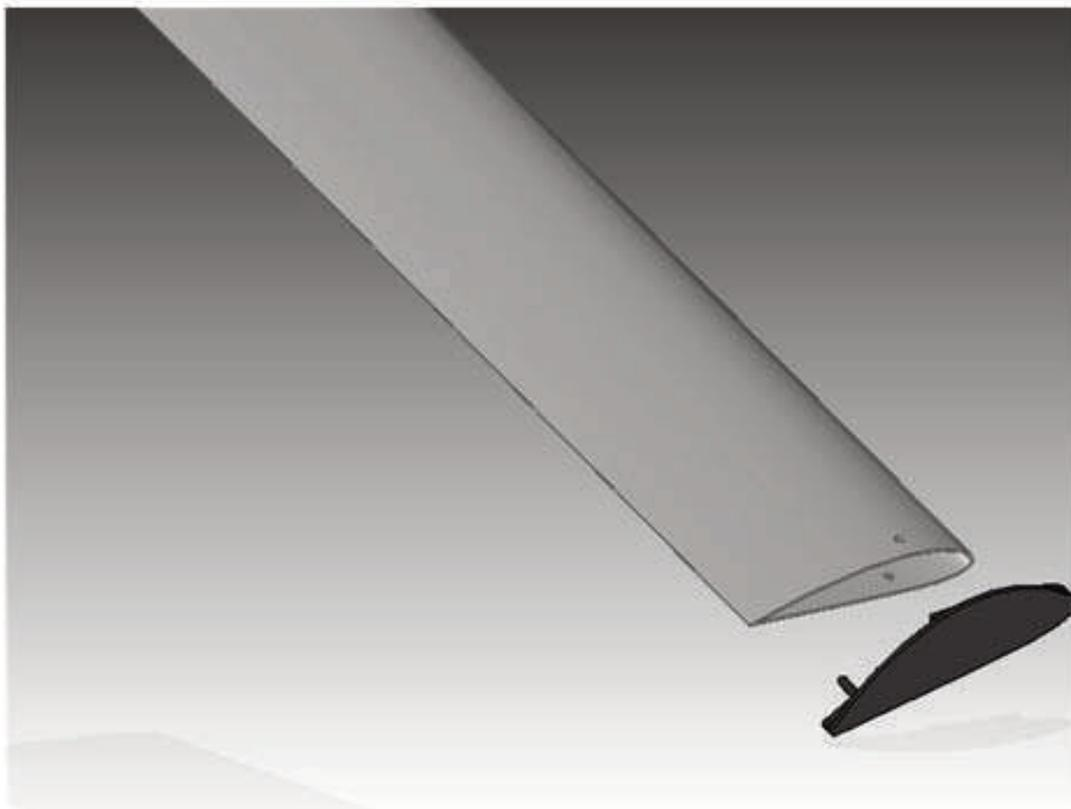
*POSITIONNER LA PARTIE TERMINALE DE LA PALE DANS LE LOGEMENT DE LA PALE
